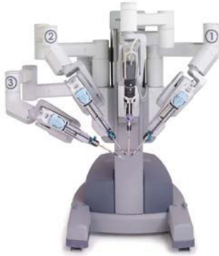
Image 1. Da Vinci system for robotic assisted laparoscopic prostatectomy [1].
