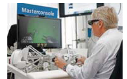
Fig.6. Operator working remotely using haptic device [www.waataat.weloved.com]
