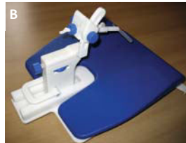
Image 3. MR-compatible tools A Manipulator for neurosurgery [4] B Prostate biopsy device [8]
