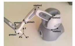
Fig.5. PHANTOM Omni Haptic Device with 6 DOF [www.cooperativehaptics.com]
