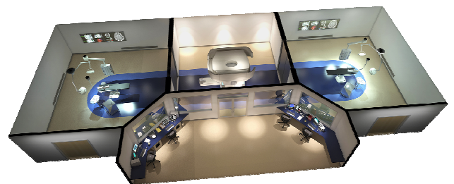
Figure 4: IMRIS IGP suite with two operation rooms and a movable MRI in the middle [15]
