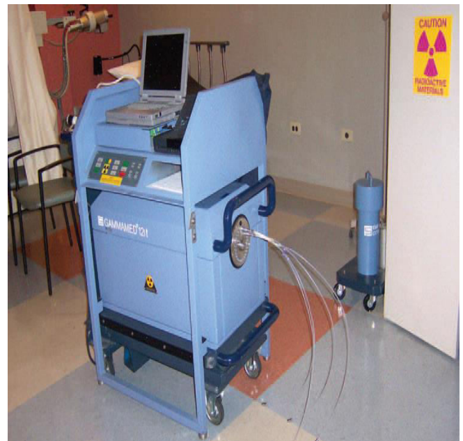
Fig3. High-dose rate brachytherapy units are remote after loading devices that use an iridium-192 source
