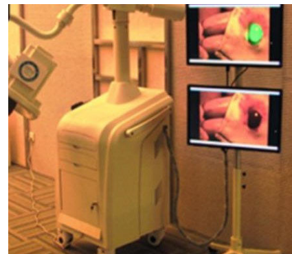
Fig.10. Surgical navigation system GXMI Navigator from the Institute of Automation, Chinese Academy of Sciences [13].
