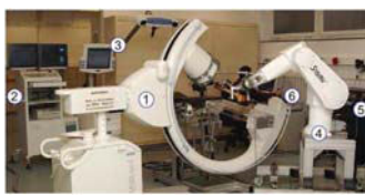
Fig.7. View of 3D Telesurgery set up where operator is sitting away from source of radiation. 1. Fluoroscopy device, 2. Fluoroscopy workstation, 3. Surgical navigation system, 4. RX 90 Robot, 5. Robot controller unit, 6. Controller PC [3]
