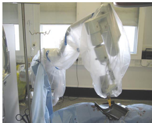
Fig6. The Intrabeam system An X-ray source is placed in the breast wound; an electron generator and accelerator are held by an articulated robotic arm. Only the shaft of the applicator can be seen; the tip of the device is in the breast tissue. A tungsten-impregnated polyurethane sheet is used to localise irradiation.
