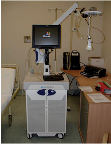
Figure 9: An example of equipment for superficial and interstitial hyperthermia (BSD 500 hyperthermia system) operating on microwaves of 915MHz.
