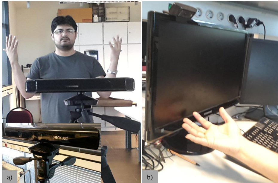
Figure A.1: a) First Context (IIKT-GP): Kinect camera is oriented in front of the subject for hand gesture and posture recognition. b) Second Context (IIKT-AR), webcam is adjusted in front of the subject in a tilted manner (i.e., 45 orientation) for AR scenario.
