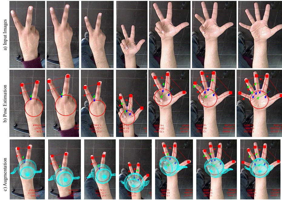
Figure 7.6: Results of content augmentation on image sequences. a) Original images b) Patch detection and camera pose estimation. c) Augmentation of 3D objects (i.e., kettle) on the hand posture.
