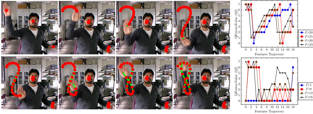
Figure 5.7: Gestural action when the subject is drawing Gesture ‘8’ using Bezier descriptor ( N = 20 ). In the sequence, Bezier points (marked as red points) are presented whereas the graphs present extracted quantized features with trajectories. Upper graph shows the features of detected Gesture ‘8’ whereas in lower graph, no gesture is detected Gesture ‘-1’.
