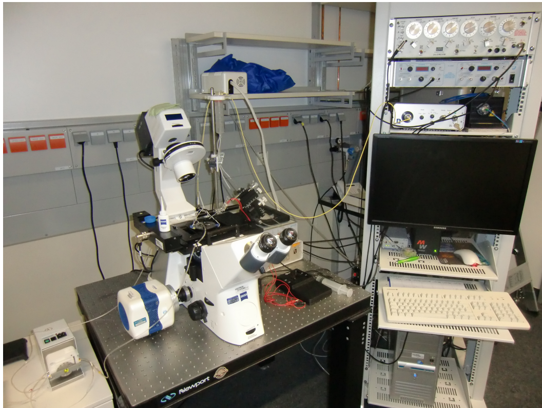
Figure 82: The WF setup that was established by the group Molecular Physiology. The major components are the inverted microscope Zeiss Axio Observer, the EMCCD camera Photometrics Evolve 512, and the light source Sutter Instrument Company LAMBDA DG-4. Electrical stimulation is provided by a manual micro-manipulator at the stage of the microscope in connection with the GRASS S48 stimulator on top of the rack on the right. Extracellular solution is provided by the ISMATEC perfusion device on the left.
