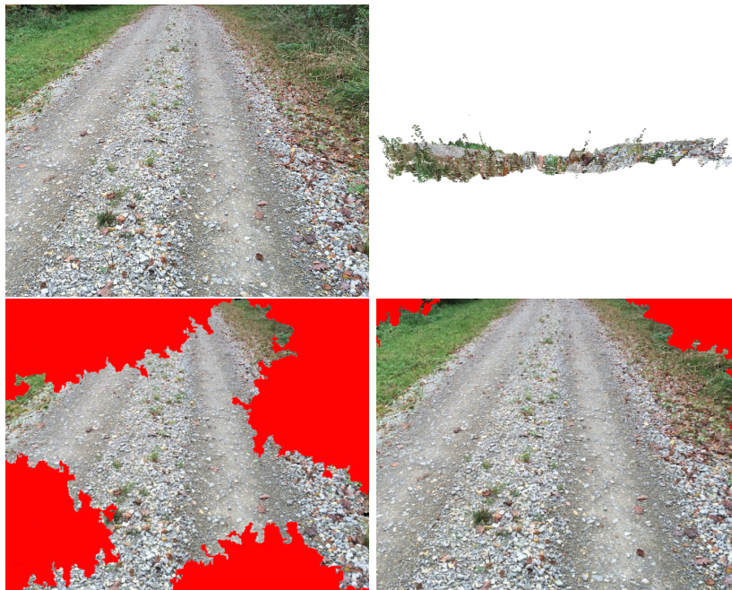
Figure 6.12: Segmentation results for rough terrain navigation. (a) Left input image. (b) Side view of the 3D reconstruction. It can be seen that the surface is quasi-planar, but not strictly planar. (c) Result for strictly planar segmentation. Many parts of the road are incorrectly labeled as obstacles (red). (d) Segmentation result of our method with correctly segmented obstacles on the side of the road (top left and top right). Image source: [HERBON et al., 2015b]
