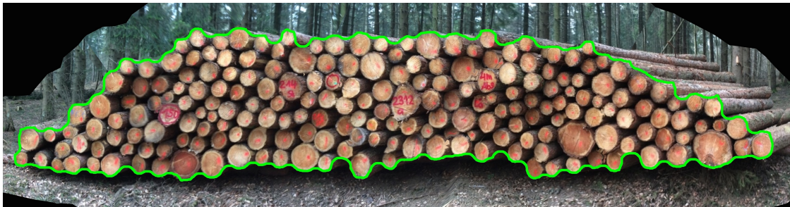
Figure 2.8: Contour volume V_c measured through a concave hull (green). The front area of the wood pile A_s is multiplied with the defined length l to obtain the contour volume V_c .
