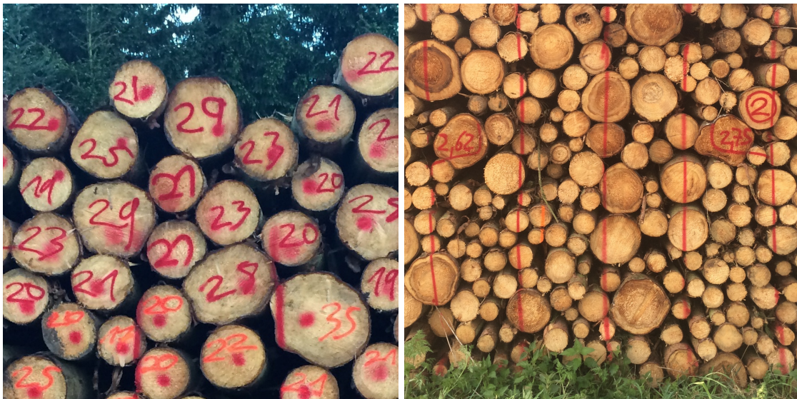
Figure 2.9: Manual surveying methods. (a) Complete midpoint diameter inventory. All diameters in [cm] are written on the wood log faces. (b) Section volume method for industrial wood. Sections of equal width are used to determine the average height of the wood pile and the height in [m] is indicated with spray paint.
