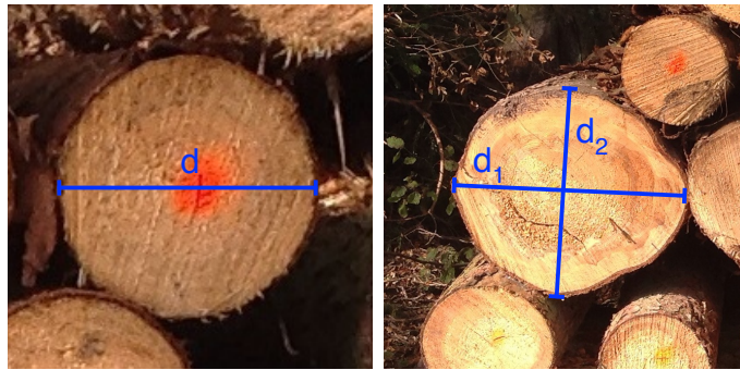
Figure 2.10: Orthogonal diameter measurement. (a) Pure horizontal measurement of the diameter for wood logs with d < 20\text{cm} , (b) orthogonal measurements for wood logs with d \geq 20\text{cm} . Image source: HAWKwood [HERBON, 2014b]
