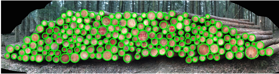
Figure 2.7: Solid wood volume V_s measured by accumulating the diameters (green). The cumulated area of the log faces A_s is multiplied with the defined length l to obtain the solid wood volume V_s .
