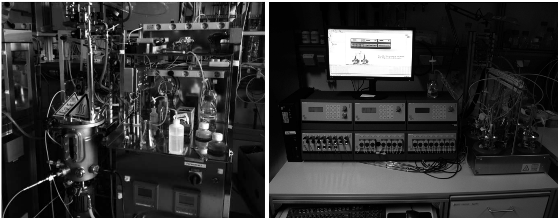
Figure 2.2.: Single bioreactor (left) with a 7 liter vessel and parallel bioreactor system (right) with up to 4 \times 750 ml fermenters.
