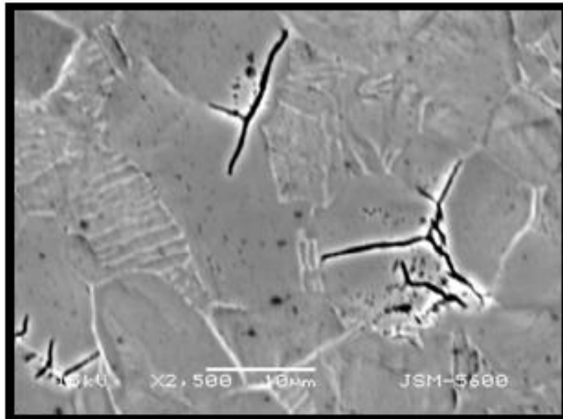
Figure 2-12: Hydrogen induced cracks along the \alpha phase boundaries in duplex Ti alloy, in the areas where hydride tend to form [120]
