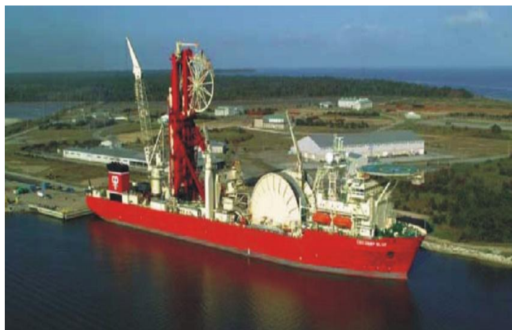
Figure 1-1: A marine vessel for welding and placement of the SMSS pipelines for the oil and gas transportation industry
