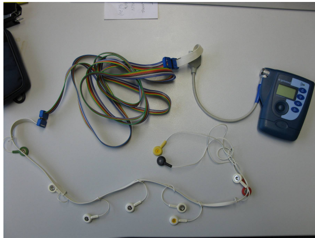
Figure 4.1.: Holter ECG (CM3000-12, Getemed, Germany) with extended cables for the usage inside a 3T MR scanner room. Electrodes were placed in a Mason-Likar 12-lead ECG configuration (see Section 2.1.2).
