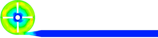
Figure B.10: Velocity at blade passage plane, 2.5 L/min, 3500 rpm
