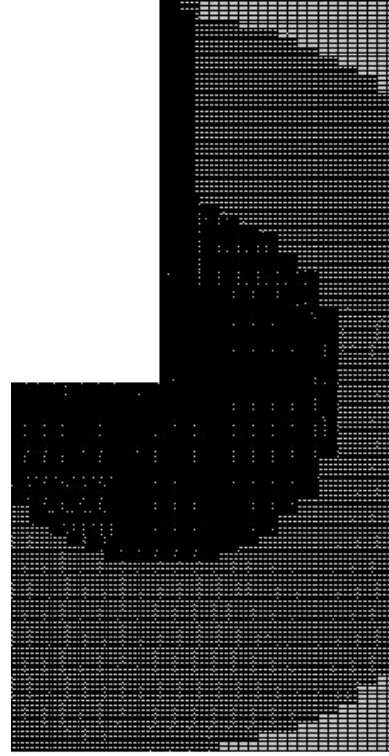
Figure 3.4: Zoom on the mesh at the end of the central tube (sudden expansion)
