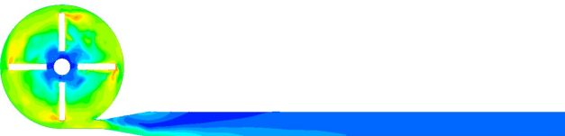
Figure B.14: Velocity at blade passage plane, 7.0 L/min, 3500 rpm
