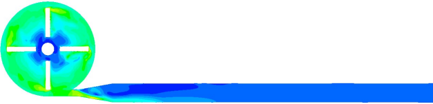
Figure B.12: Velocity at blade passage plane, 6.0 L/min, 2500 rpm
