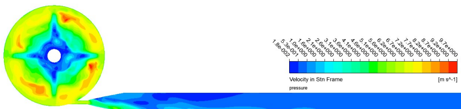
Figure B.47: Velocity at 6 L/min and 3500 rpm, upper gap
