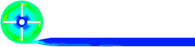
Figure B.9: Velocity at blade passage plane, 2.5 L/min, 2500 rpm
