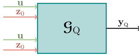
Figure 3.11: Structure of a first-order DAE system with a quadratic output.
