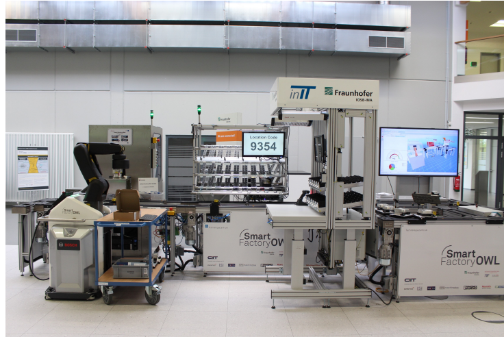
Figure 5.3: Customisable Production System demonstrator in the SmartFactoryOWL from the AutoS 2 research project
