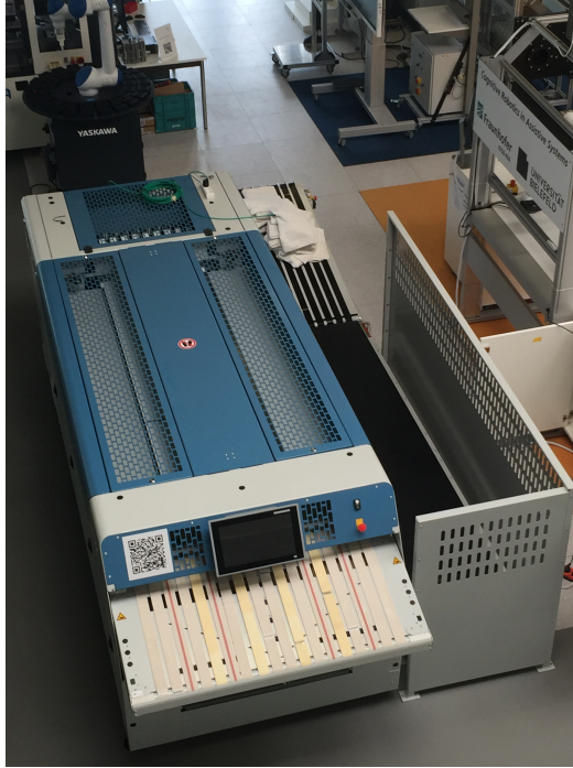
Figure 5.2: Industry-grade towel folding machine in the SmartFactoryOWL from the ADIMA research project
