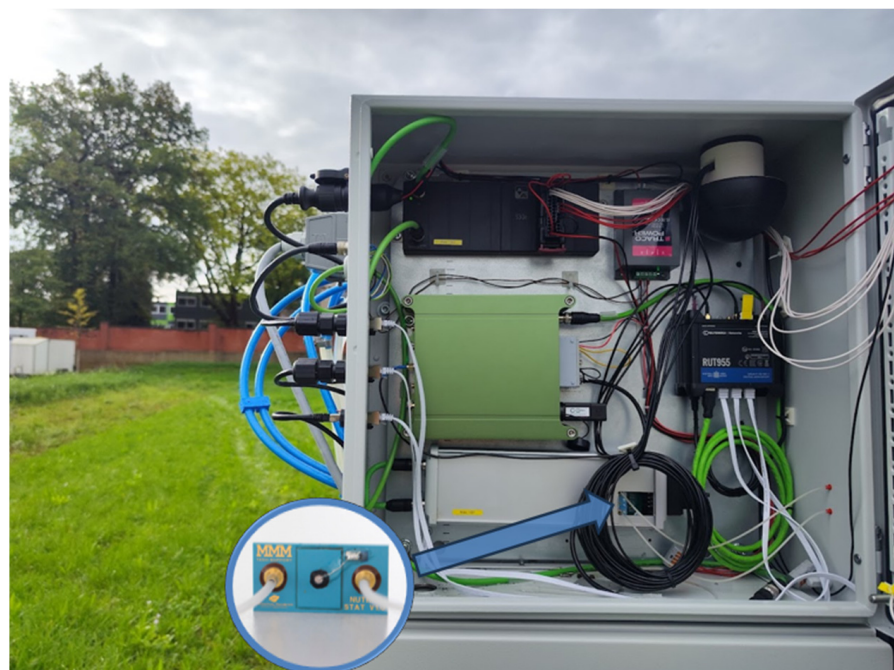
Figure 10. System integration of ISFET measurement system in soil application.
