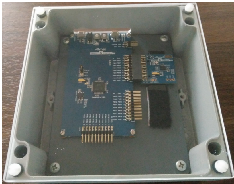
Figure 10.6: 9 DOF Sensor Setup of the electronics in a robust housing.
