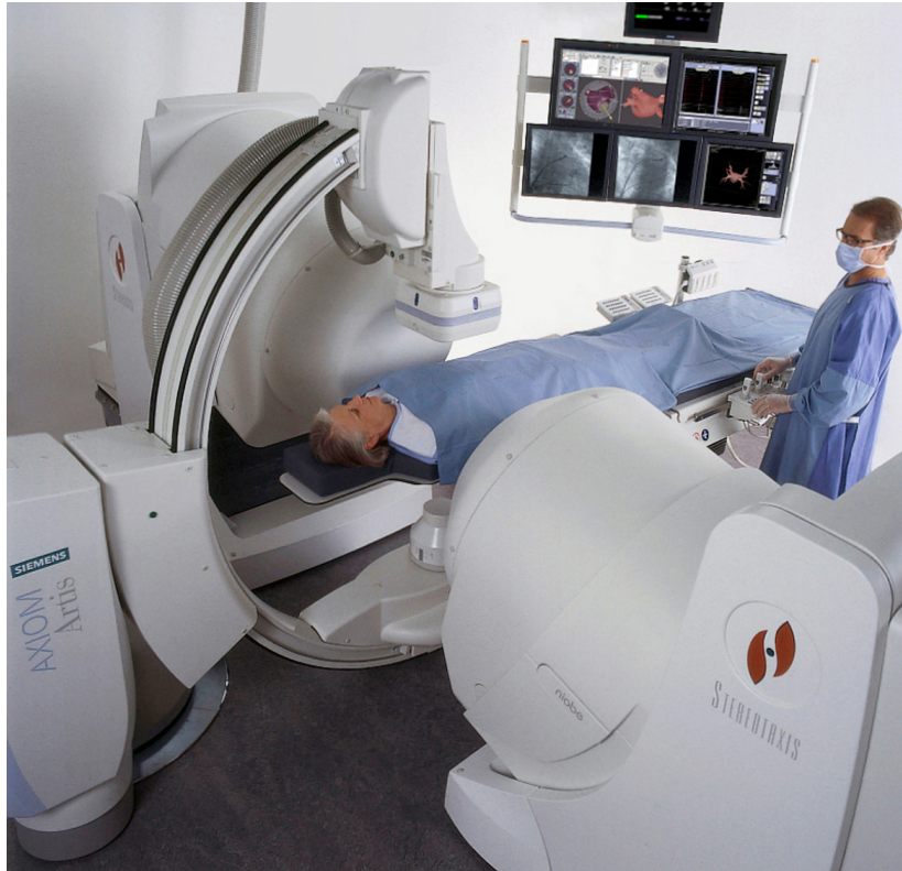
Figure 1.5: Stereotaxis Niobe EM system combined with Artis zee cone-beam CT system. (Hea17)
