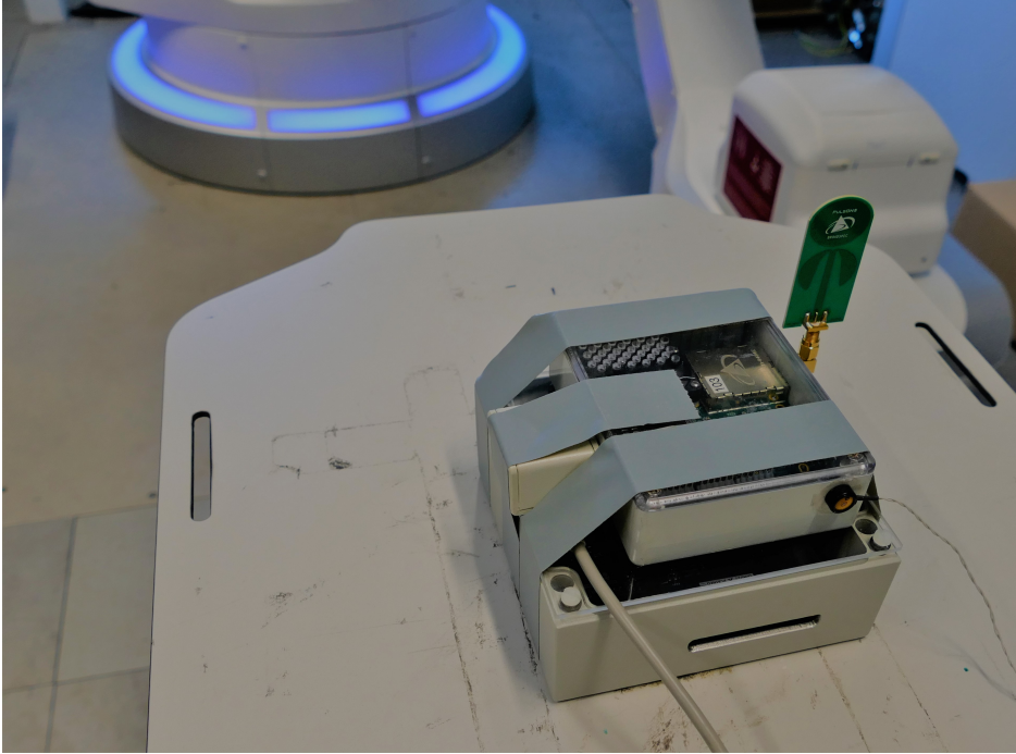
Figure 10.7: Combined sensor setup on patient table in medical environment comprising the P410 UWB module, both IMUs and an Optotrak optical marker.
