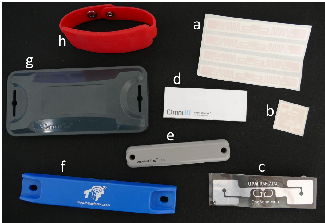
Figure A.1: Various implementations of RFID transponders are available on the market. It starts with printed tags with different antenna designs in a, b and c. Other exemplars like d and e are fabricated in plastic material to be more robust. Massive housing of the RFID antenna can be found in f and g to be able to use the tags on metallic surfaces. RFID tag f is embedded in a flexible and wearable wristband.
