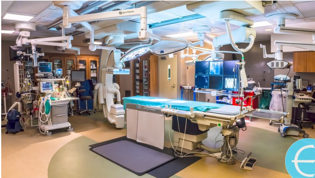
Figure 1.1: Typical hybrid operating room setup with ceiling-mounted cone-beam CT system Artis zee, Siemens patient table, large ceiling mounted display, ceiling supplies with OR-lights and other devices positioned on movable trolleys. (Inc17)
