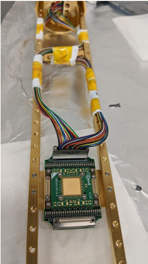
Fig. 3.12 QBoard mounted on a sample puck: (a) The QBoard sample holder attached to the probe that mates with the MXC flange through the FSE mechanism. The wires are thermalized by attaching them to the probe with Teflon and kapton tapes. (b) QBoard containing a sample with multiple devices and all contacts bonded. The 48 DC contacts available on the QBoard allows for a high throughput in the testing of devices at low temperatures. The aluminium wire bonding acts as the main source of thermalizing the sample at very low temperatures. Hence multiple bonds, if possible, would be encouraged.
