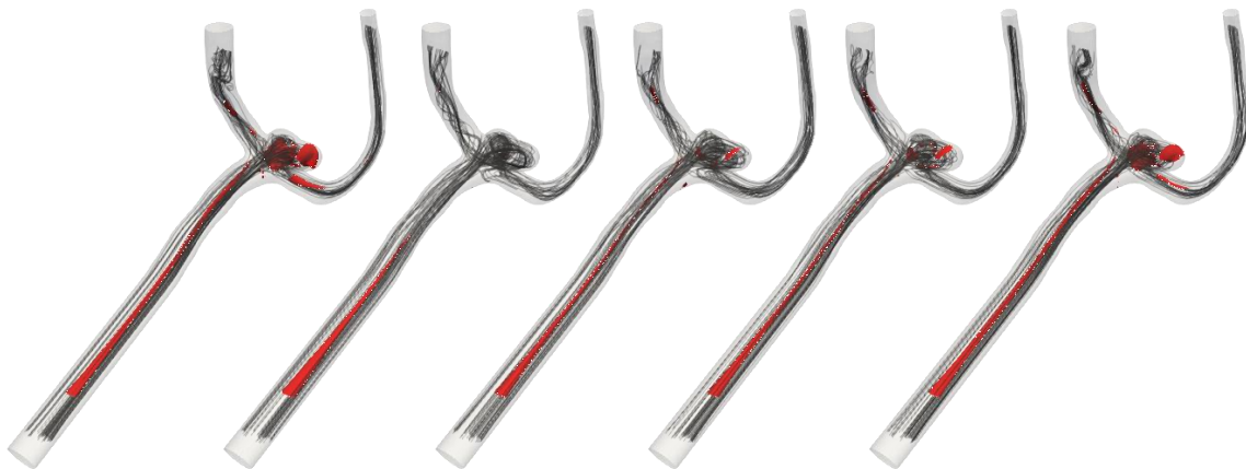
Figure 4.7: Streamlines at different times over a cycle for the first patient-specific configuration. From left to right: 0.1, 0.3, 0.5, 0.7 and 0.9 s. The red iso-surfaces show regions with shear rates below 100 \text{ s}^{-1} .
