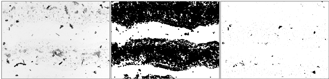
Figure 27: Exemplary visualization of the dust segmentation according to ST4\_DUST , shown for an aged CLSM intensity image ( t = 30 w). From left to right: aged grayscale fingerprint image (including settled dust); segmented area PM\_DUST for dust investigation (dilated two times, black: masked fingerprint region, white: background region used for dust observation); segmented dust according to ST4\_DUST\_IMG_n (binarized for better visualization).
