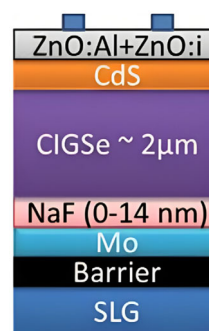
Figure 1. Schematic layer stack of the CIGS solar cell. The CIGS absorber layer with a thickness of about 2 μm is doped with Na by depositing a NaF precursor layer onto the substrate, before CIGSe evaporation.
