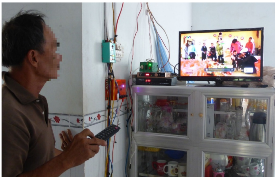
Figure 9. A low-voltage television set is the central appliance in the household system
