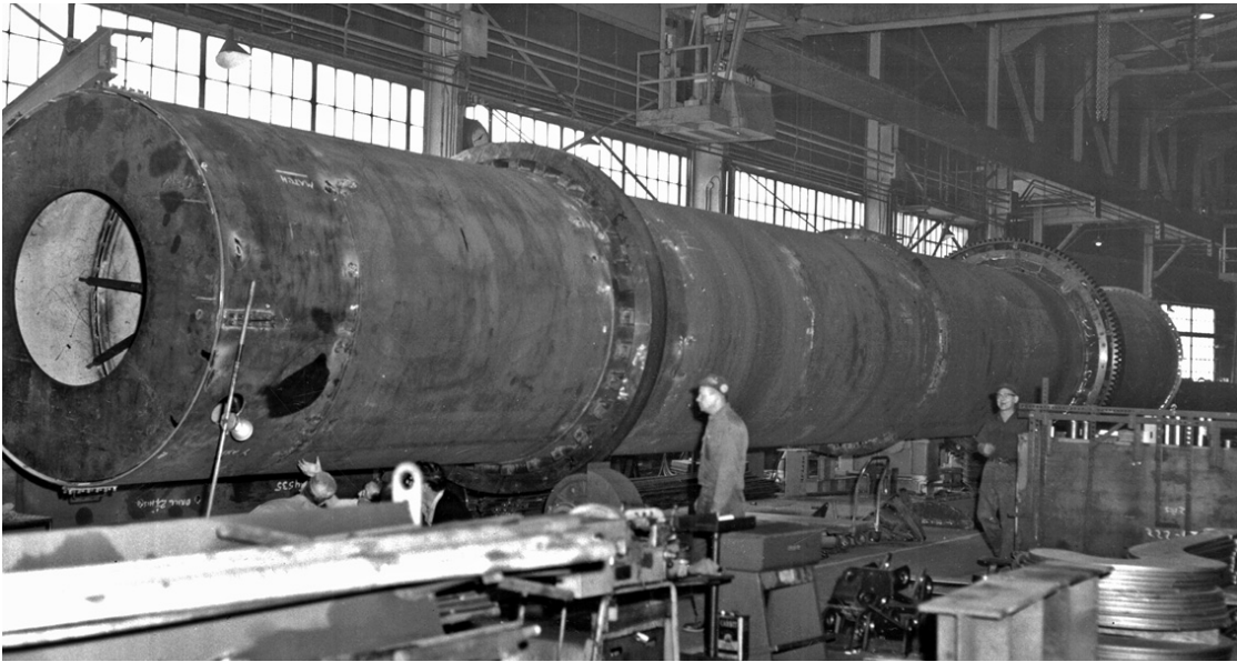
Figure 1.4: Direct heat rotary dryer during manufacture [18]
