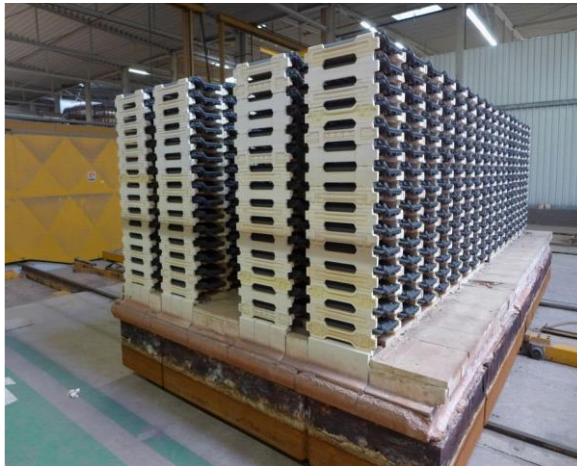
Figure 3-1 Actual setting of roof tiles and cassettes on kiln car (Photo: BMI Technical Services GmbH)
