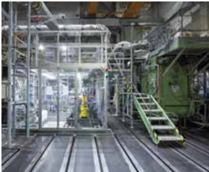
Figure 3: Low viscosity fuel module (left) and single cylinder research engine (right)
