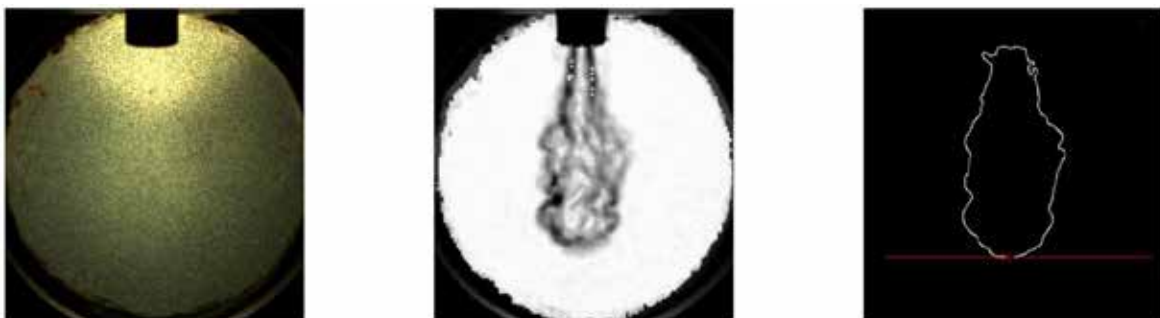
Figure 3: Overview of the postprocessing steps – Raw image, BOS image, binarized jet borders
