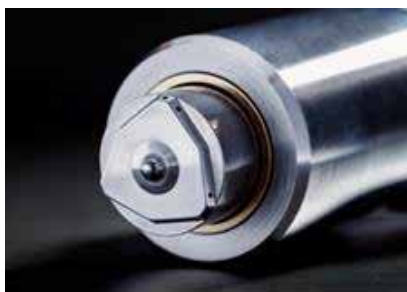
Figure 9: HPDF nozzle with 3 concentric Methanol needles and one central diesel needle
