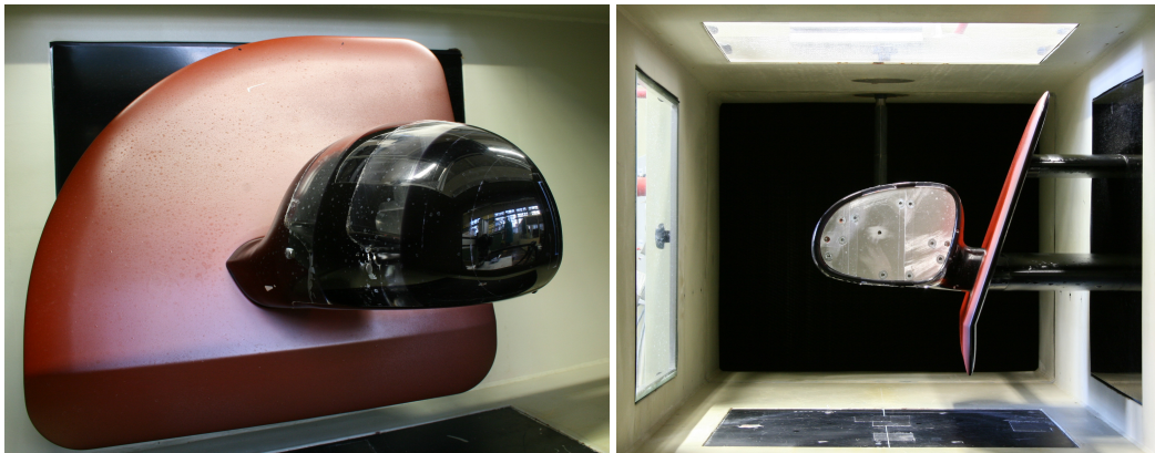
FIGURE 4.6: Wing mirror model mounted in the test section of the wind tunnel; side view (left) and view in upstream direction (right)
