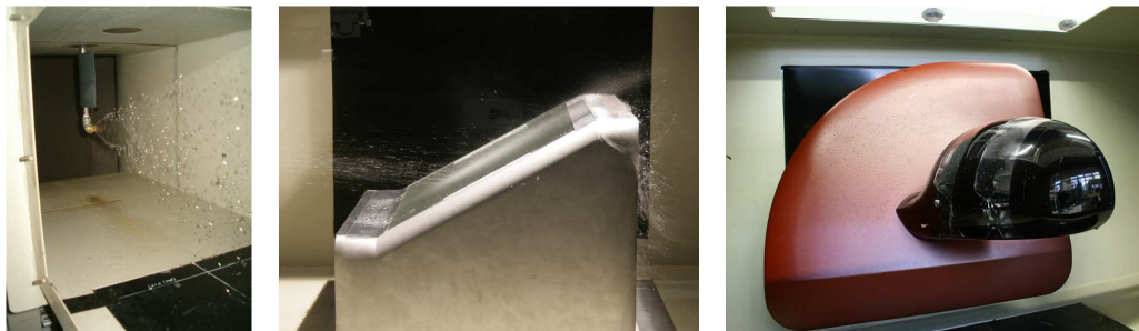
FIGURE 4.1: Experimental configurations: K0 empty test section (left), K1 generic windshield geometry (middle), K2 rear view mirror geometry (right); pictures of windshield and rear view mirror by B. Faßmann
