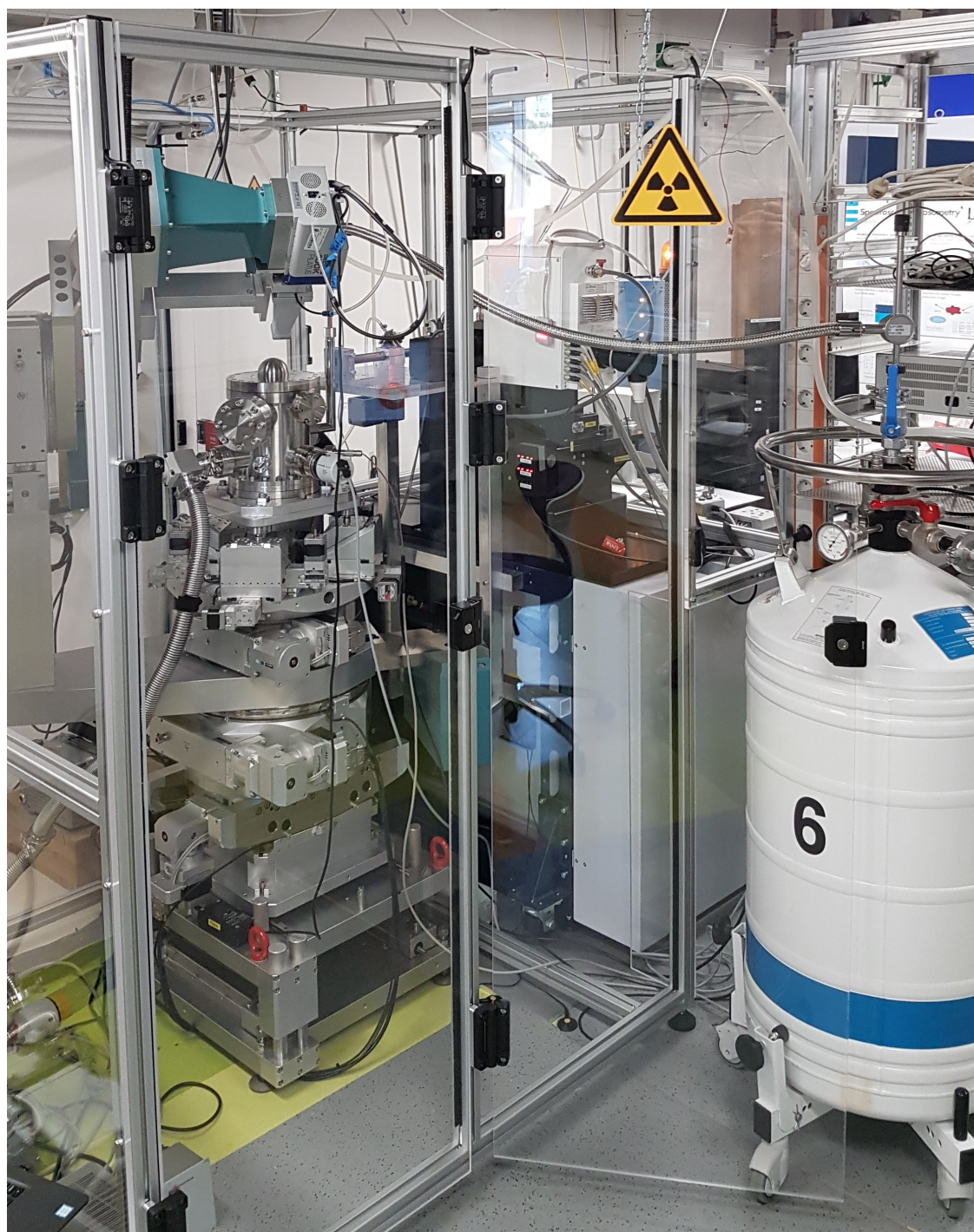
Figure 2.10: Photograph of the six-circle diffractometer used in this work, equipped with a Ga jet X-ray source and a cryostat for temperature-dependent XRD measurements.
