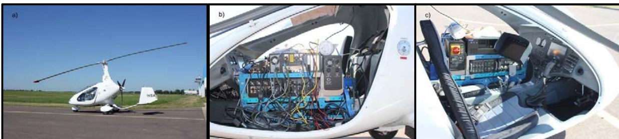
Figure 1: Gyrocopter D-MHSA hosted by Anhalt University of Applied Sciences and applied for research and teaching remote sensing of the environment within the institute of geoinformation and landsurveying. a) presenting
