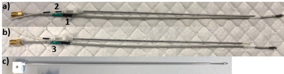
Figure 5.21: Preparation of the temperature sensor using the catheter as a guide for positioning in the liver tissue. a) Catheter tip is parallel to the applicator slot center. b) Measuring tip of the temperature sensor is parallel to the applicator slot center. c) Catheter rod for cleaning the guide.
