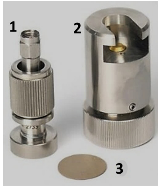
Figure 5.7: High-temperature probe option 101 of N1501A dielectric probe kit: 1. High-temperature probe. 2. High temperature short. 3. Conductive disk. [59].
