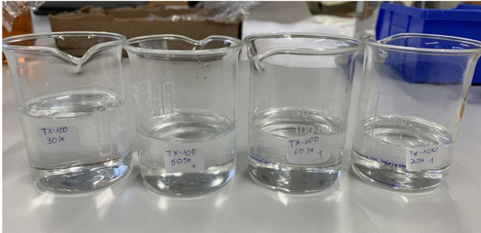
Figure 5.11: Phantoms with 30 %, 50 %, 60 % and 70 % concentration of TX-100.
