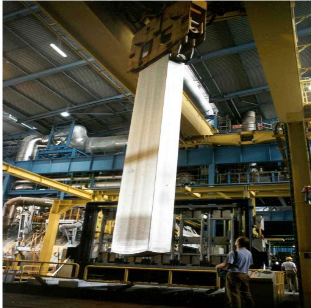
Figure 1.3: Aluminum strand after casting (courtesy:NOVELIS INC.)
