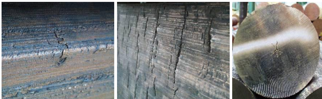
Figure 1.5: Typical cracks in the continuous casting of Copper alloys
