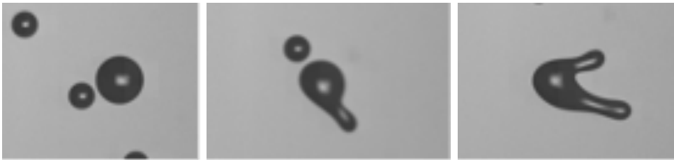
Figure 4.2: Example of one big droplet colliding with two small droplets
