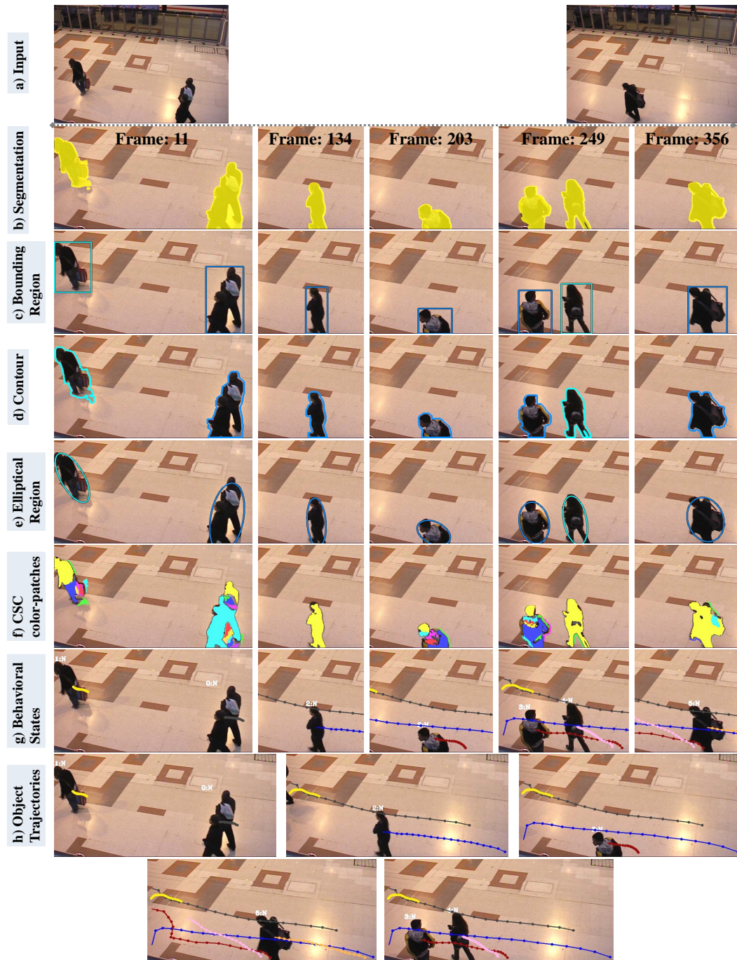
Figure A.4: shows results on PETS2006 [1]. a) input sequence, b) the extracted objects from segmentation, c) the computed bounding region over the detected objects, d) contour of the objects, e) ellipse around the object which are used to compute the ellipse histogram, f) CSC color-patches of each detected object, g) and h) demonstrate the results tracking and behavior understanding approach.
