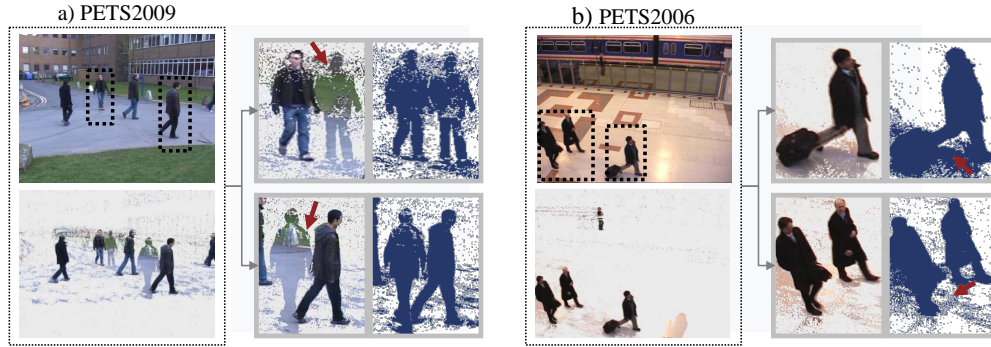
Figure 2.3: presents the segmentation outcome of non-recursive approaches on PETS2006 [1] and PETS2009 [3] datasets. a) shows segmentation result of median filtering approach [20] where the learning time delay caused a ghost object which is not presented in the actual scene. b) shows the segmentation result of the approach [21] where over segmentation is observed along with additional noise in the final foreground detection.
