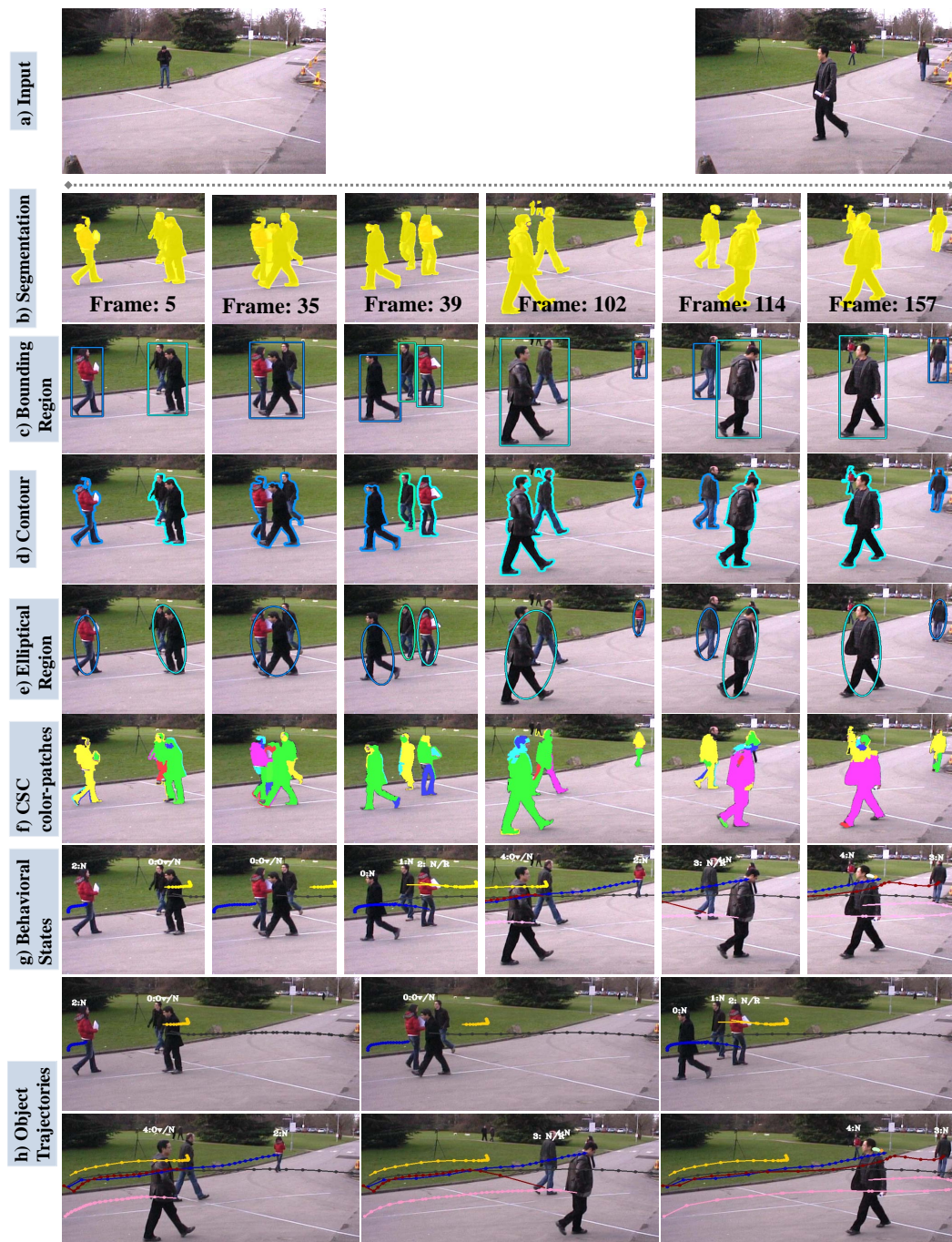
Figure A.6: shows results on PETS2009 [3]. a) input sequence, b) the extracted objects from segmentation, c) the computed bounding region over the detected objects, d) contour of the objects, e) ellipse around the object which are used to compute the ellipse histogram, f) CSC color-patches of each detected object, g) and h) demonstrate the results tracking and behavior understanding approach.
