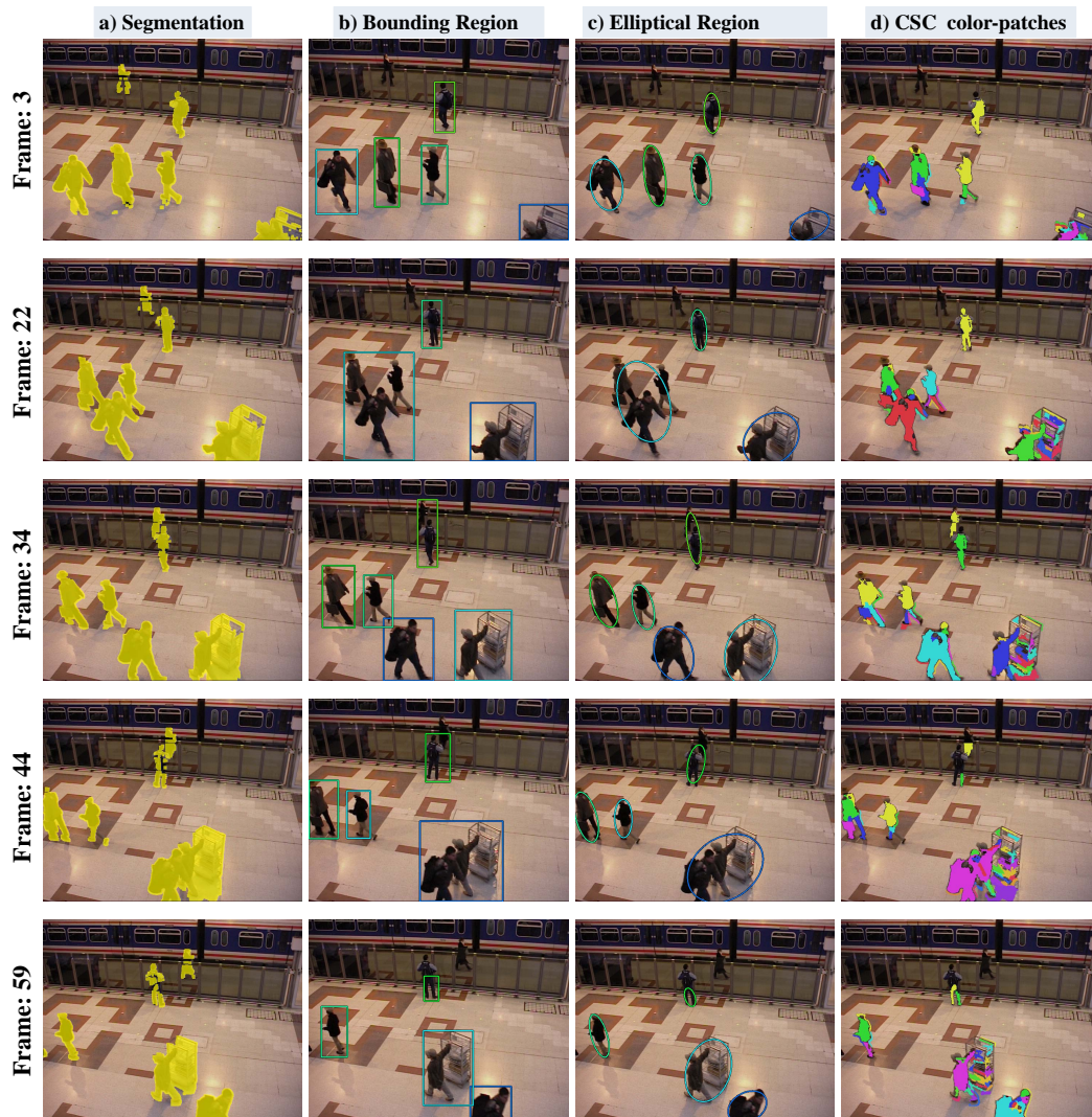
Figure A.8: shows results on PETS2006 [1] dataset. a) the extracted objects from segmentation, b) the computed bounding region over the detected objects, c) ellipse around the object which are used to compute the ellipse histogram and d) shows the CSC color-patches of each detected object.
