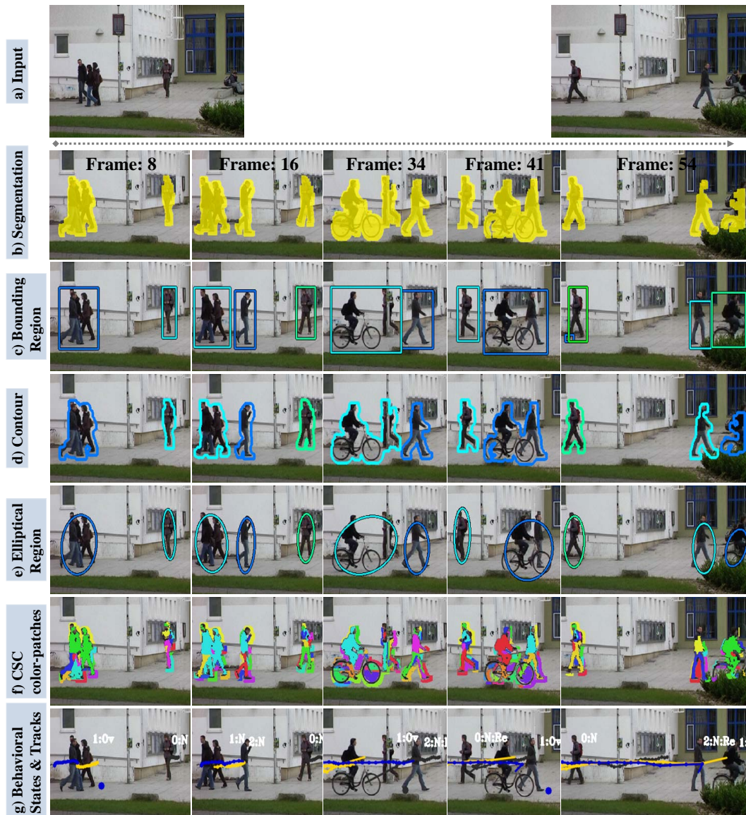
Figure A.7: shows results on IESK dataset. a) input sequence, b) the extracted objects from segmentation, c) the computed bounding region over the detected region objects, d) contour of the objects, e) ellipse around the object which are used to compute the ellipse histogram, f) CSC color-patches of each detected object, g) demonstrates the results tracking and behavior understanding approach.
