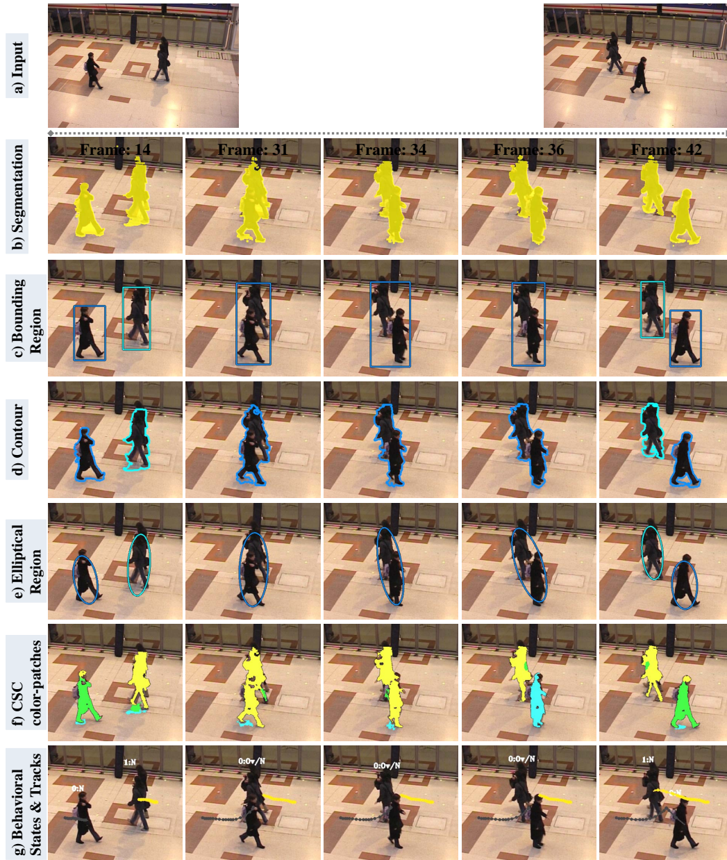
Figure A.5: shows results on PETS2006 [1]. a) input sequence, b) the extracted objects from segmentation, c) the computed bounding region over the detected objects, d) contour of the objects, e) ellipse around the object which are used to compute the ellipse histogram, f) CSC color-patches of each detected object, g) demonstrates the results tracking and behavior understanding approach.
