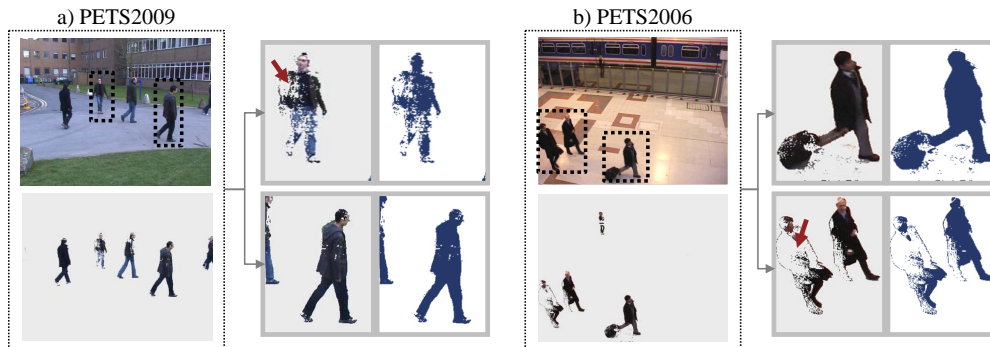
Figure 2.4: presents the results of recursive techniques on PETS2006 [1] and PETS2009 [3] datasets. a) shows the segmentation result of approximated median filtering approach [22] where an object is fragmented into parts due to slow pace. b) shows the segmentation results of the approach [26] where under segmentation (i.e., empty regions of holes in objects) is observed due to the constant region in the object.
