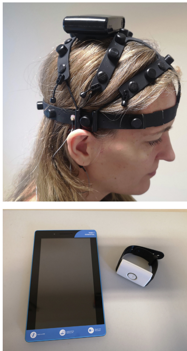
Fig. 1. Fourier One™ (F1) mobile EEG system; left: headset with amplifier electronic box; right: tablet and event marker.
