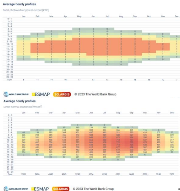
Figure 3: Power and Solar radiation data of the installed station.
