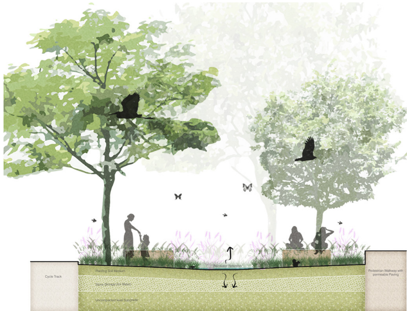
F.5.9 Conceptual Sketch Section of Bio Retention Areas
