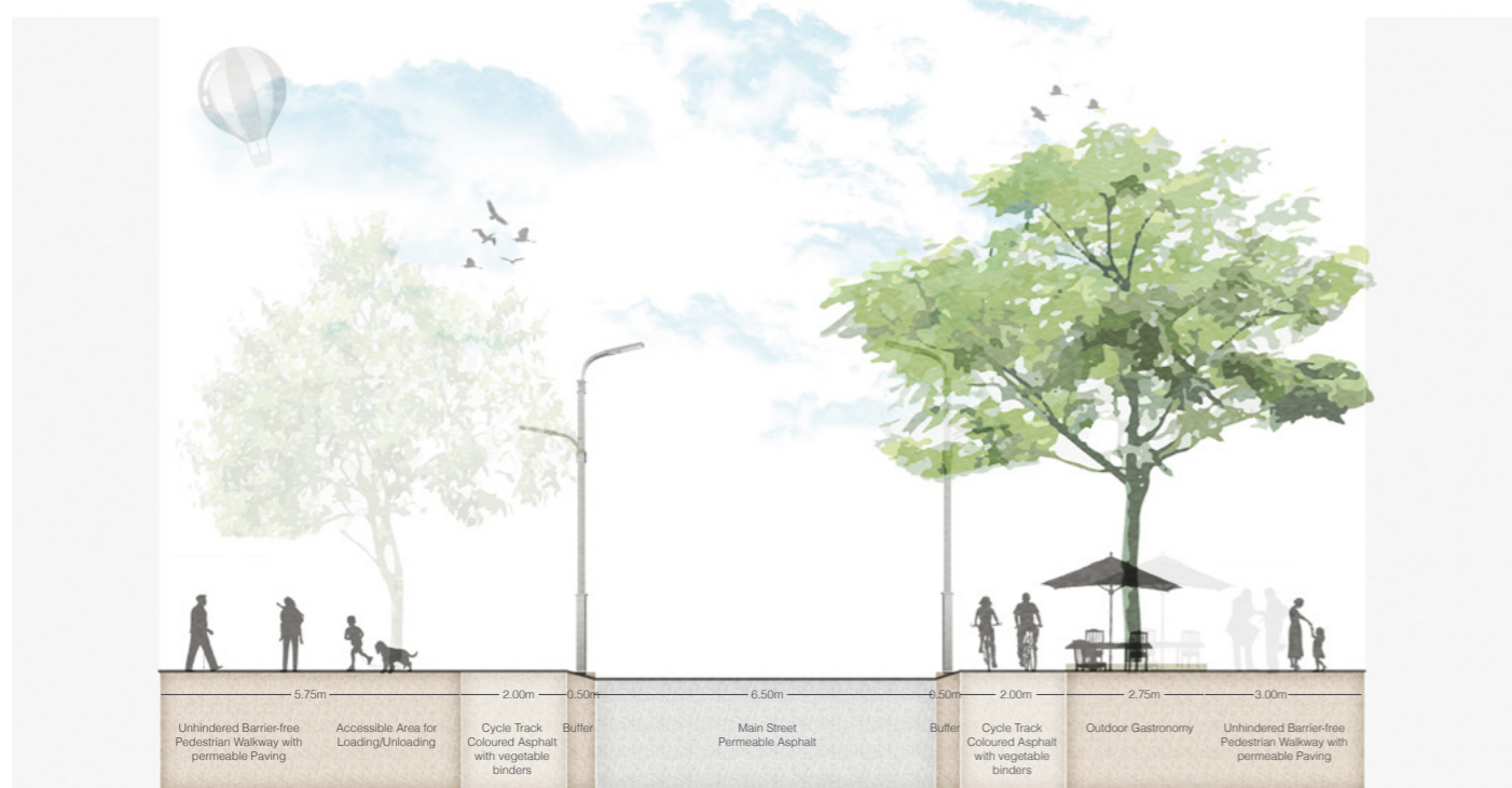
Section DD Typical Section through Schweizer Straße
