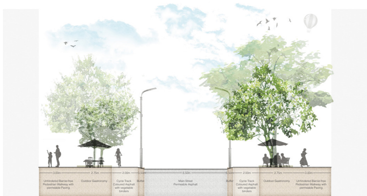
Section CC Typical Section through Schweizer Straße
