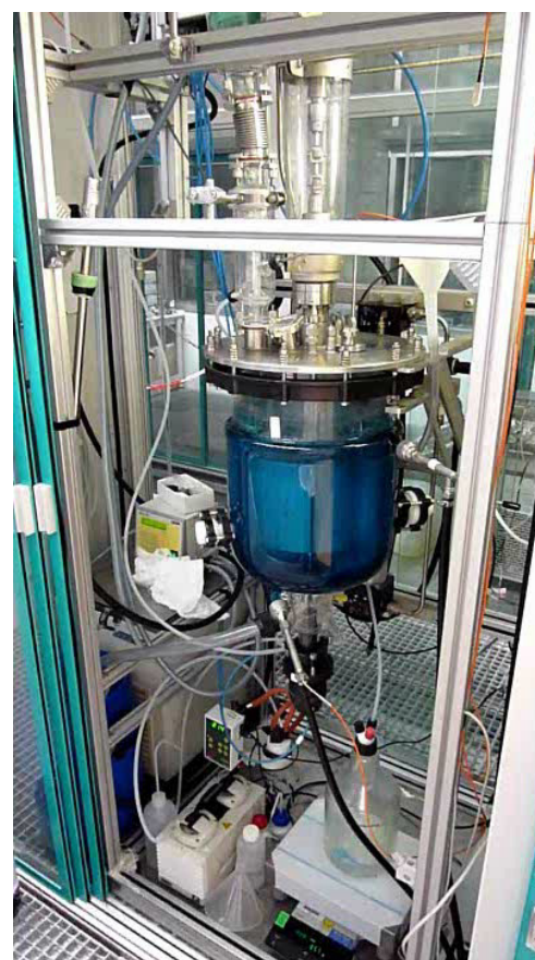
Figure 5.36 Batch-crystalliser equipped with solvent reflux and distillate balance. The draft tube inside the vessel is visible.
