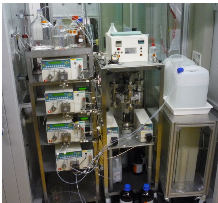
Figure 5.35 Preparative scale multi column chromatographic separation unit. Four identical columns are installed (centre of figure) and connected to a multiport valve, which operates from top. The pumps for feed, extract, raffinate and eluent are placed on the left side.
