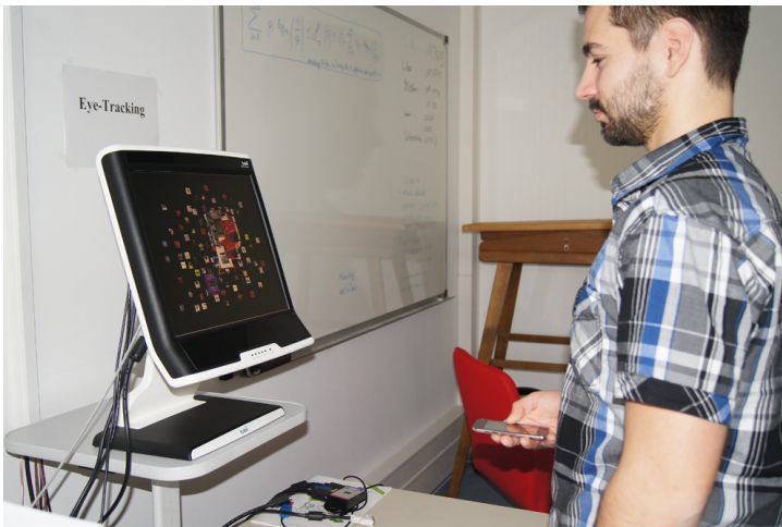
Figure 64: Photograph from [pub:20] of a participant standing in front of the Tobii T60 eye tracker to interact via gaze and an iPod Touch with GazeGalaxy .
