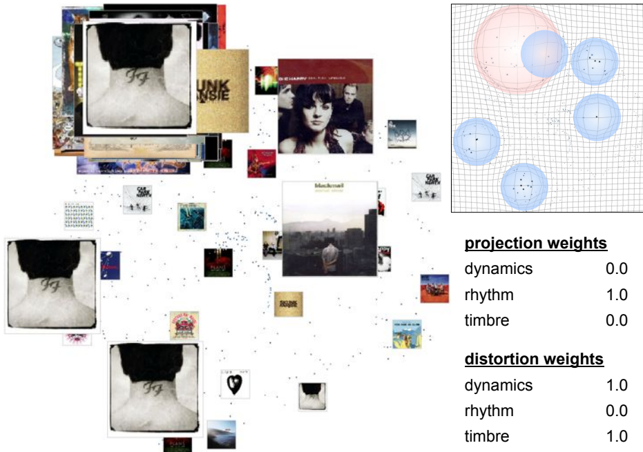
Figure 60: Using a bisociative SpringLens setting to explore a music collection. Top: MusicGalaxy visualization (inverted color scheme for print). Bottom right: corresponding lens distortion resulting from (user-controlled) primary focus (red) and (adaptive) secondary lenses (blue). Bottom left: facet weights for the projection and distortion distance measures (values adaptable).
