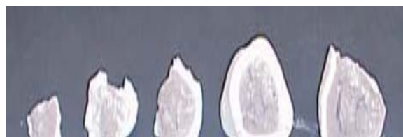
Figure 1.6: Cross section of unburned lime particles [9].
