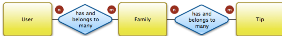
Figure 6.4.: Entity-Relationship diagram of the basic, access-controlling relation between the main entities User, Tip and Family. In contrast to common practice, only an existing direct or indirect relation between the instances grants access to it. Access control for a Tip instance to a particular User is implied by a relation of both instances to at least one common Family.
