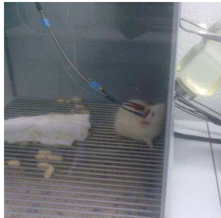
Fig. 6. Recording chamber with an animal inside. The rat is connected through a ribbon cable to the swivel; the tube connecting the injector with the microsyringe is also appreciated. The animal had free access to water and food.
