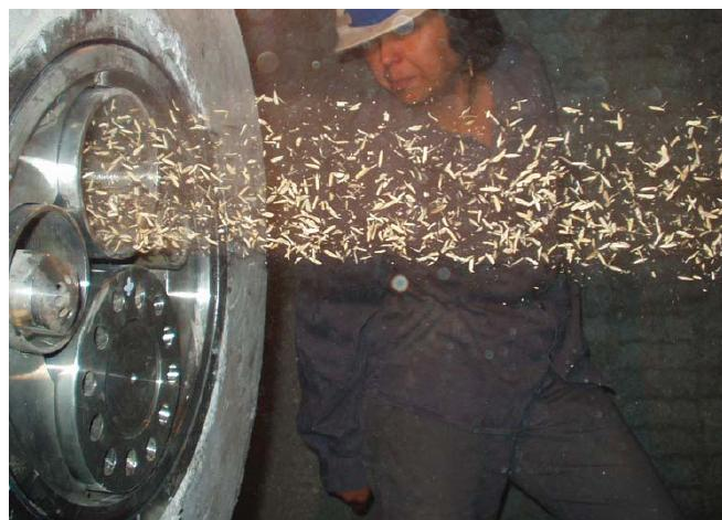
Figure 2.11: DUOFLEX burner using waste fuels, [7].
