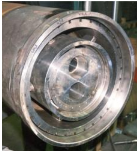
Figure 2.23: A typical Polysius burner [40].
