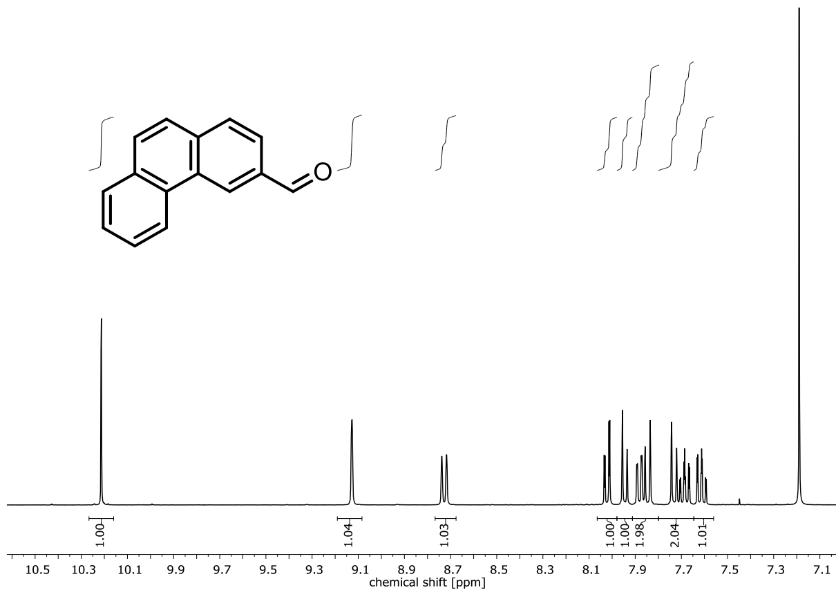
Figure 8.80: ^1\text{H-NMR} spectrum of phenanthrene-3-carbaldehyde.
