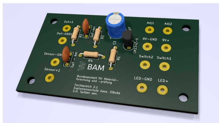
Figure B.4.: PCB for the calorimeter, available under https://aisler.net/p/EWHXKDFG
