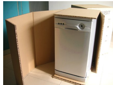
(a) Honeycomb composition of an aircraft wing (b) Paper honeycomb panels used for packaging
