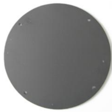
Figure 3.18: Back side of aluminium sheet for spray quenching
