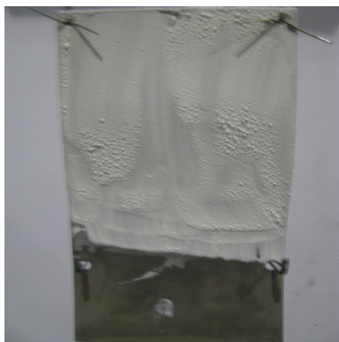
Figure 3.3: Surface of KS 83 coating after heating into furnace at 600 °C
