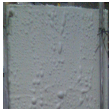
Figure 3.4: Surface of KS 82 coating after heating into furnace at 600 °C
