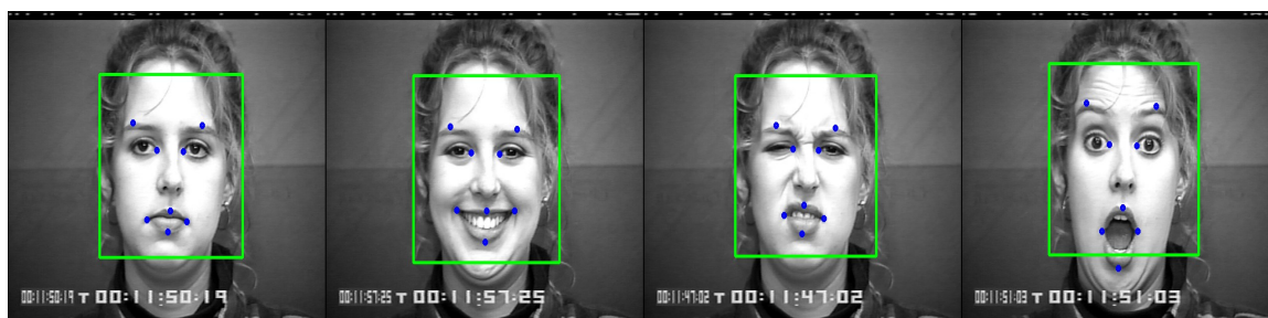
Figure 7.10: The face cropping is invariant to the expression (mouth and eyebrow deformations). A same face expresses four expressions (neutral, happiness, disgust, and surprise), while the cropping has a fixed distance to the eyes center. (Images from Cohn-Kanade database, © Jeffrey Cohn.)
