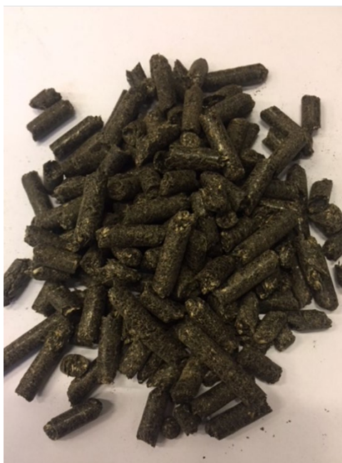
Figure 3.2: The sunflower seed shell casings pellets, a more oil-rich type of pellet, produced from the residue after sunflower oil production.
