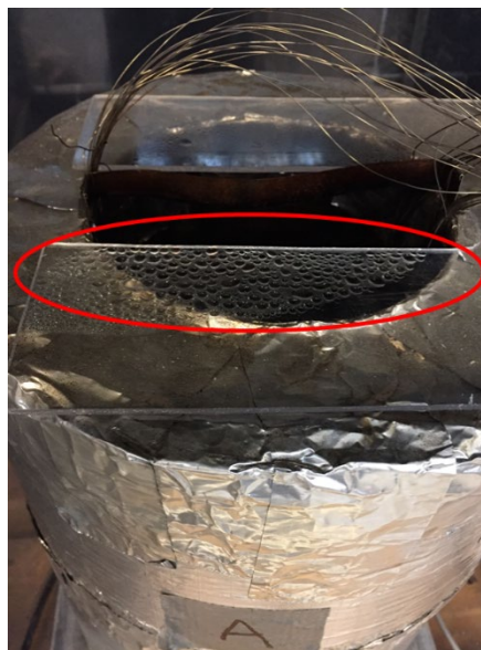
Figure 6.15: Condense on plastic coverage of the steel pipe. The condense is marked with a red circle. The condensate dripped down on and affected the top layer of the sample.
