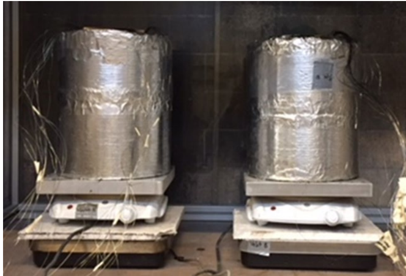
Figure 3.9: The two experimental setups in the lab. The pipe to the left was used for wood pellets, and the pipe to the right was used for oily pellets. The two assemblies are placed inside a cabinet, which is closed at three sides: left, right and rear sides. The cabinet has an opening at top with ventilation above. This ensures the same external conditions, and the experiments were run in parallel.
