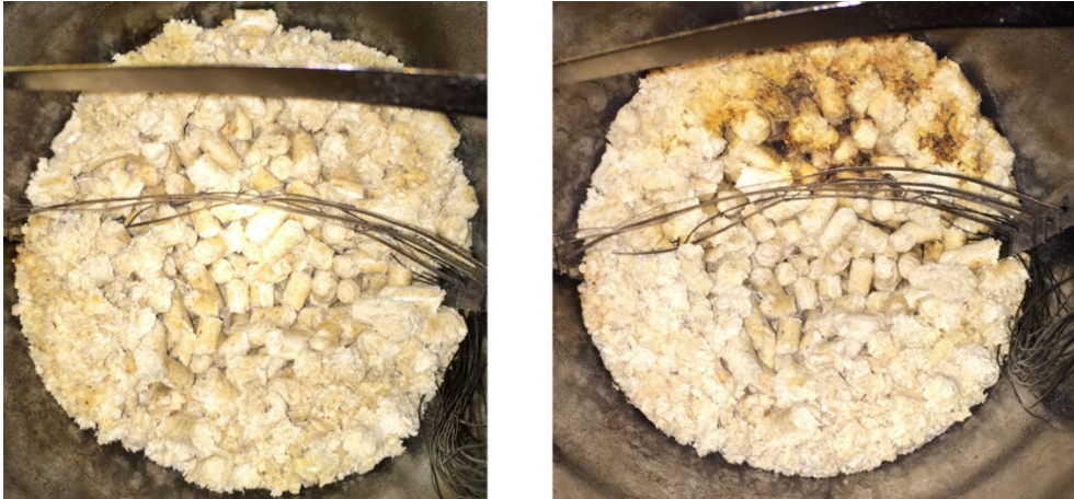
Figure 4.17: Physical changes of the wood pellets. The pellets were affected by the heating of the sample and the pyrolysis front. The pellets along the pipe wall have broken apart, and in the picture to the right there has been a color change from beige to light brown.
