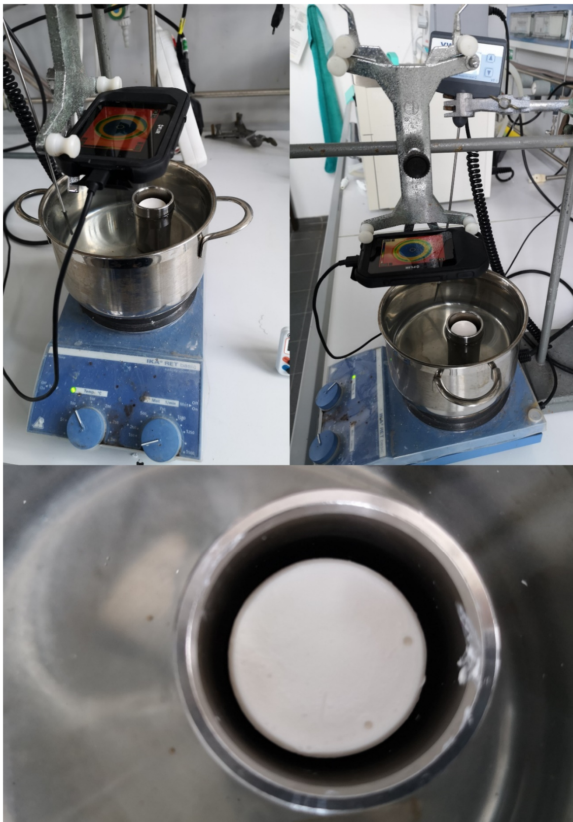
Fig. S4.2 Pictures of the construction of the thermal imaging experiment. The sample was cooled to 11 °C and put in a metallic vessel. The sample inside the metallic vessel was put in a water bath at 45 °C. The temperature of the sample was tracked via a thermal imaging camera every 15 s. Video files about the temperature evolution in the ss-PCMs containing 5 wt%, 10 wt%, 15 wt% and 20 wt% hBN are marked as Movie S4.1 - S4.4.
