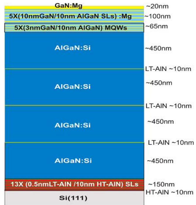
Figure 6.3.1 Scheme of the full structure for AlGa 0.9 N-based UV LED samples on Si(111)
