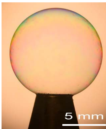
Figure 2.4: An elastomer balloon prepared by cross-linking of a LCP bubble in SmA phase.
