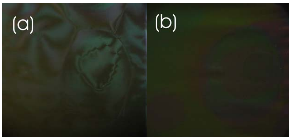
Figure 4.5: Smectic LC polymer film in the SmC* phase observed with crossed polarizers (a) before and (b) after the crosslinking.
