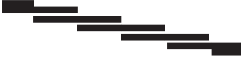
Figure 1.10: Layout of microstrip bandpass filter using half-wavelength side coupled resonators.
