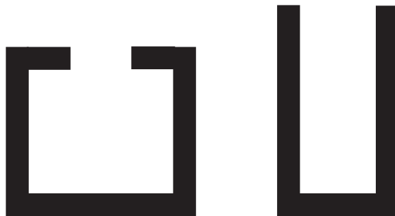
Figure 1.3: Two possible shapes of open-loop resonator.
