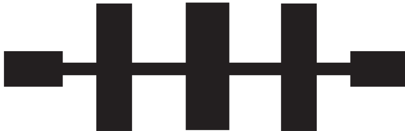
Figure 1.6: Top layout of stepped impedance microstrip lowpass filter.
