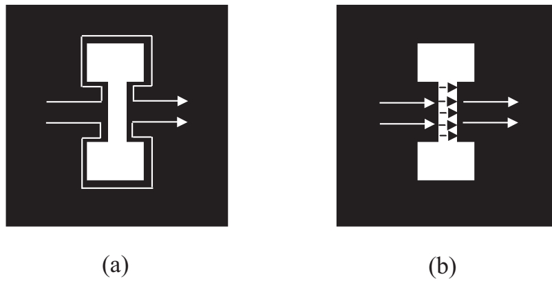
Figure 4.5: Representation for the wave propagating on the slot metallization (a) at frequency lower than the resonant frequency, (b) at frequency higher than the resonant frequency.
