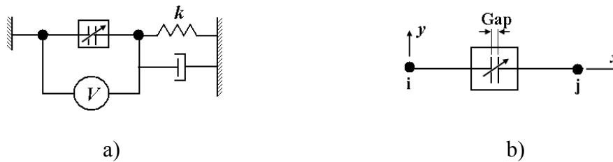
Figure 2.10: The ANSYS TRANS126 element: (a) finite element interpretation, and (b) geometry of the TRANS126 element.
