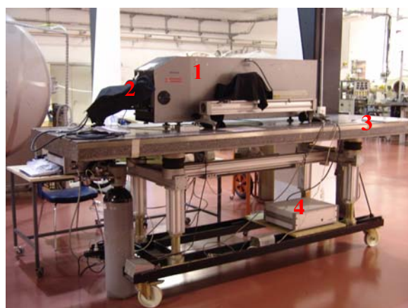
Fig.II.17. (Left) diagram of apparatus used for optical emission spectroscopy in the visible range and (right) UV-VIS high resolution SOPRA Czerny–Turner type spectrometer used in this study.
