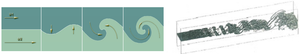
Figure 3.5: Left / Schematic of a mixing layer between two parallel flows of respective velocity \vec{U}_1 and \vec{U}_2 - development of a Kelvin-Helmholtz instability. Right / Vorticity modulus of the same type of instability obtained with Large Eddy Simulation (reproduced from Lesieur et al. [83]).
