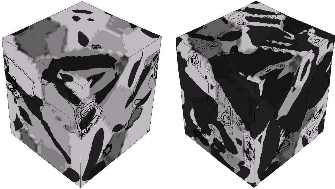
Figure 7.27: Twin spreading on the RVE, at a nominal compression strain of 3.3% and 4%. The greyscaling indicates the grain structure. The twins are the dark areas, while the accumulated basal slip is depicted by the contour lines (0 to 0.004 in the left and 0 to 0.06 in the right figure).
